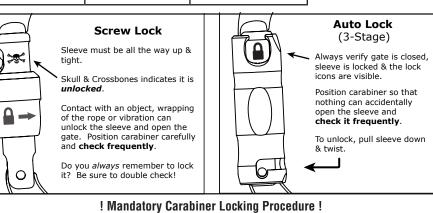
Serious accidents have resulted from unlocked carabiners. Dirt, ice, etc. can jam a sleeve. Never assume autolock carabiners lock on closing - always confirm! You may forget to lock a manually locking sleeve-always double check! You must understand how the sleeve works and know what it looks like when it is locked and unlocked.
